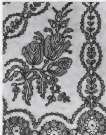
Detail of a parasol cover of imitation Chantilly lace, made on the pusher machine, from Nottingham, Eng.; in the Museum and Art Gallery, The Castle, Nottingham, Eng.
